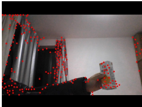
Figure 1. Shi-tomasi corner detection effect
